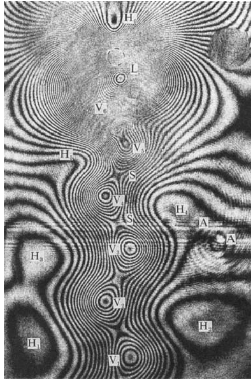
FIGURE 6. Interferogram showing near wake and far wake for Re = 80.0 , D = 3.02 mm.
